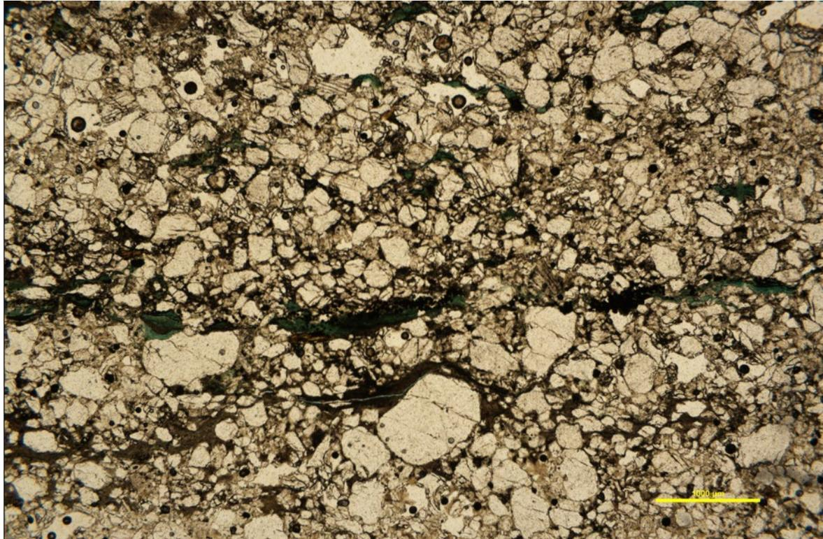
TS700-5: Poorly sorted sandstone comprises mixture of angular to subangular grains that are less than 0.1 mm long to subrounded to rounded grains that are up to 1.0 mm long. The feldspar (microcline and plagioclase) grains are most common in the smaller grain size fraction. The dark laminae running through the middle of the photomicrograph appears to be dark brown organic matter and green glauconite.
