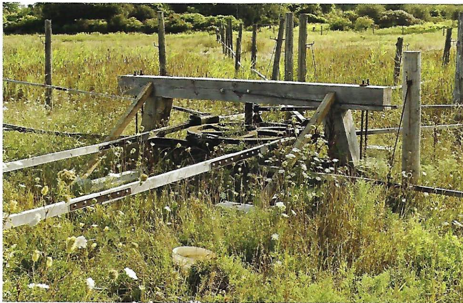
Fig. 6. Cast-iron field wheels are hubs for the jerker lines that radiate in different directions. Once common, they are now rare, and there are 12 at Fairbank Oil Fields. Photo courtesy of Carol Graham.
